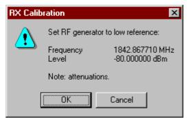
When the user acknowledges by pressing OK, the calibration with low input level is executed.
