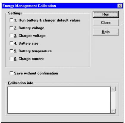
A DC power supply, a service battery and a 3–wire charger calibration cable is needed for this calibration.
