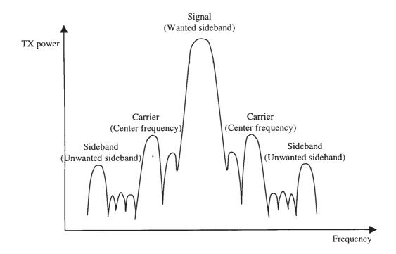
Adjust the Amplitude difference and the Phase difference stepwise until the side bands are suppressed as much as possible (Refer to the drawing above). When tuning adjust the values slowly step by step.
