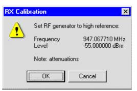
When the user acknowledges by pressing OK, the calibration with high input level is executed.
