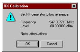
When the user acknowledges by pressing OK, the calibration with low input level is executed.
